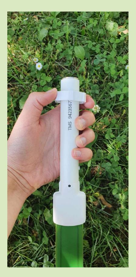
First, put on the security ring (no.1). Make sure the arrows are pointing upwards.
